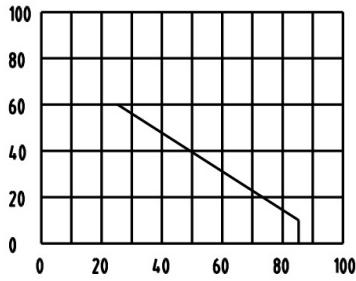
FORWARD CURRENT VS DERATING CURVE 正向电流递减曲线图
